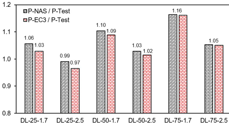
Figure 7: Comparison of test strengths and the predicted strengths
