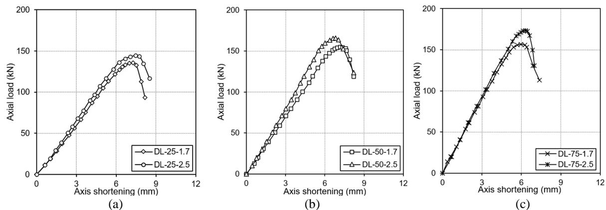
Figure 5: axial load vs. axial shortening behaviour, (a) DL-25-1.5 & DL-25-2.5; (b) DL-50-1.7 & DL-50-2.5; DL-75-1.7 & DL-75-2.5.
