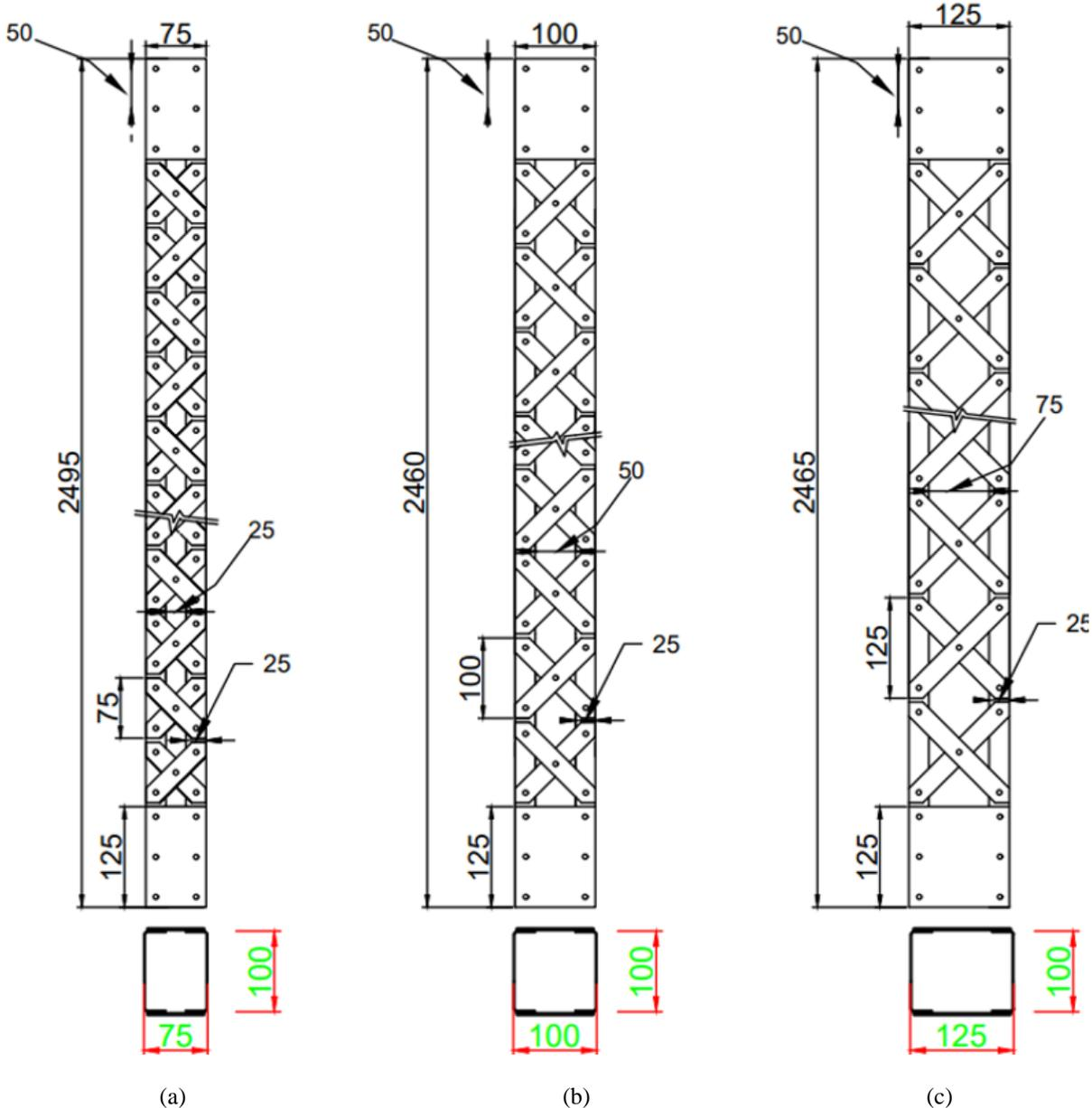
Figure 1: Longitudinal details of the test specimens, (a) DL-25-1.7 & DL-25-2.5; (b) DL-50-1.7 & DL-50-2.5; DL-75-1.7 & DL-75-2.5.
