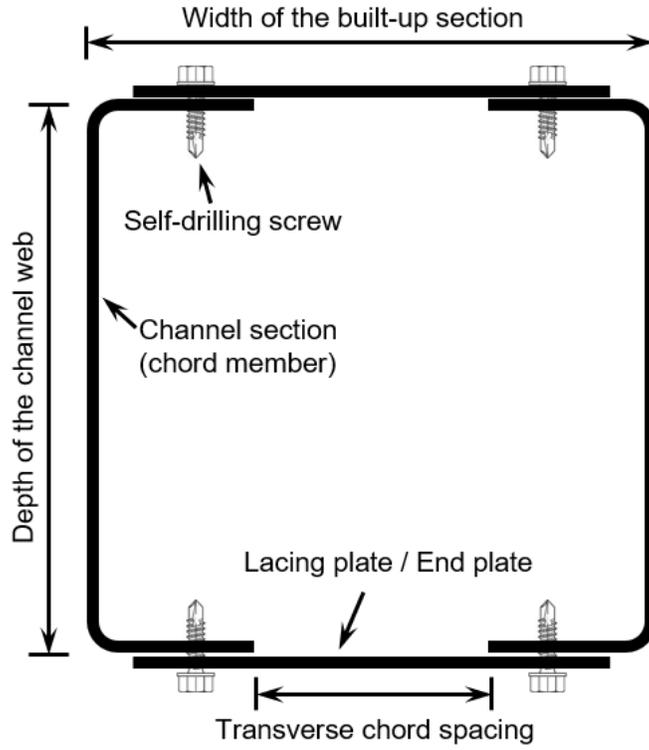
Figure 2: Cross-sectional details of the built-up column specimens
