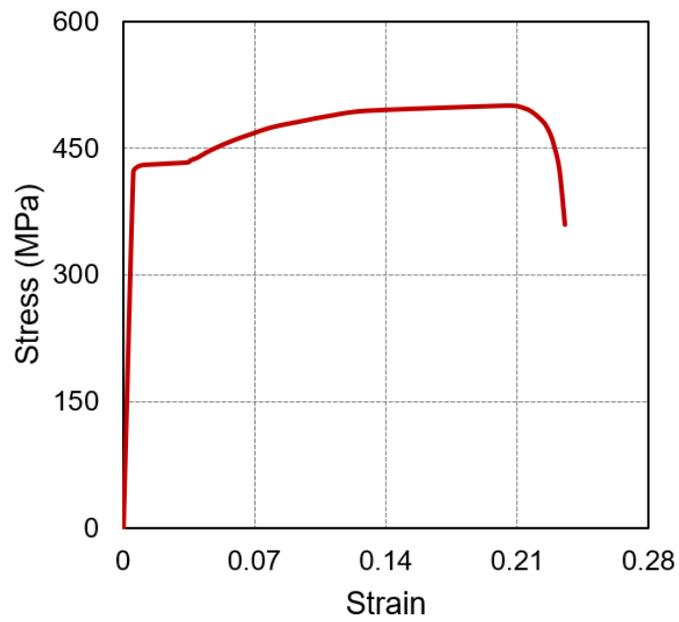
Figure 3: Typical stress-strain plot of the coupons
